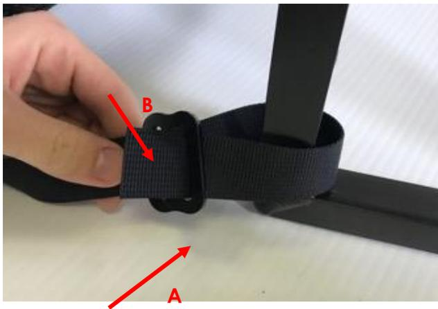
3 : Loop back around the frame and insert the strap into A.
