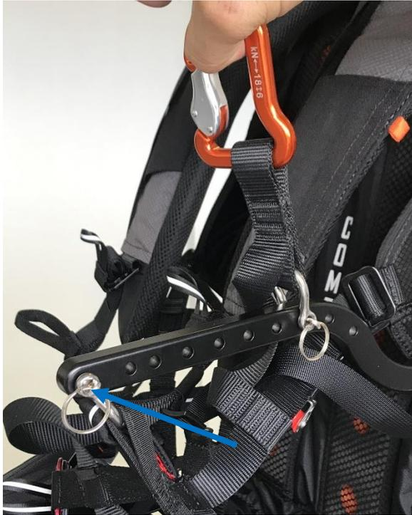
8 : Fix the shackle at the end of the arm, in the last drilling (blue arrow).
