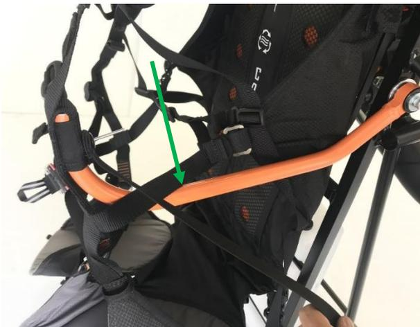
3 : Position the arm as shown. Put the end of the arm in the designed slot. Take care to pass under the strap shown by the green arrow. Position the blocking strap and add a rivet to fix the whole.
