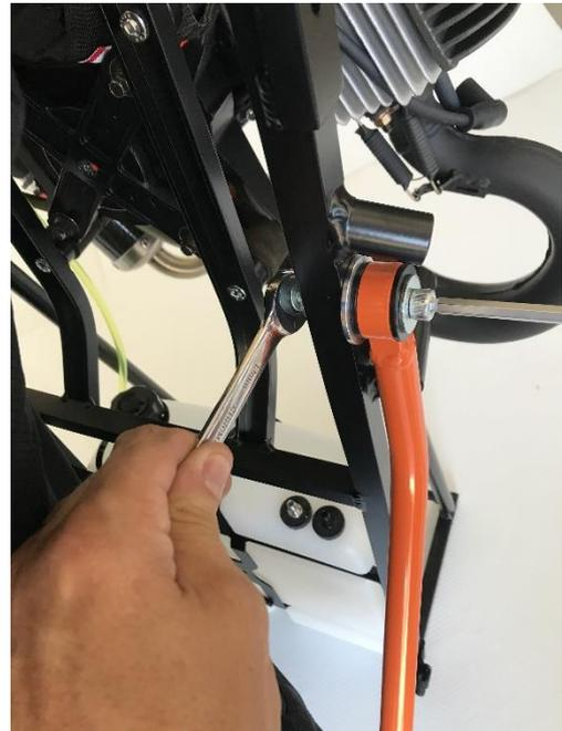
2 : Position the arm as on the picture, then attach with the spanner and the Allen key.
