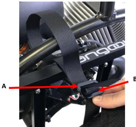
3 : Loop back around the hoop and insert the strap into A.
