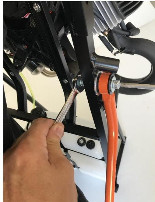
2 : Position the arm as shown, then attach with the spanner and the Allen key.
