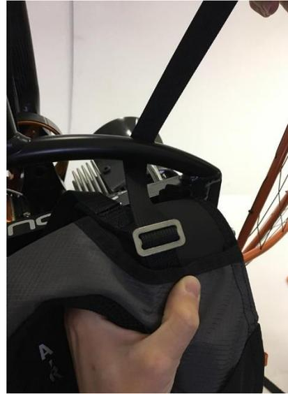
*2 : Set up the harness against the frame and pass the strap under the hoop.*
