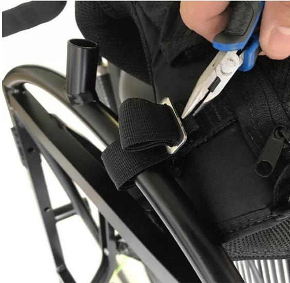
*5 : Using pliers, pull the end of the strap.*
