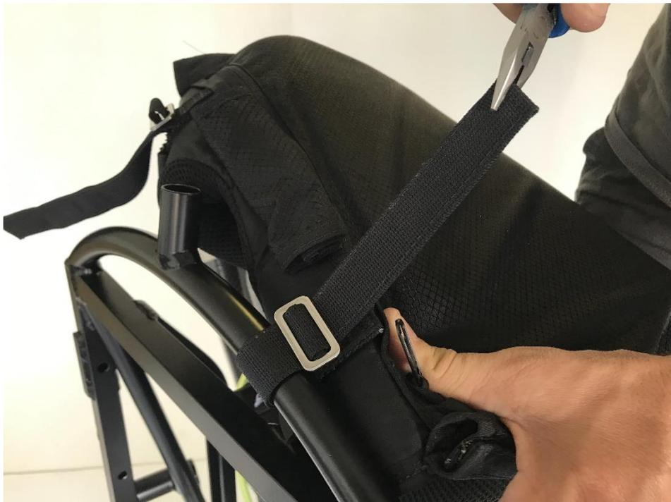
*7 : Tighten the strap snug to the fram and then rotate the harness forward.*
