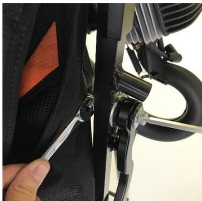
3 : Tighten with the 13 mm spanner and the 6 mm Allen key. Do it on both sides.
