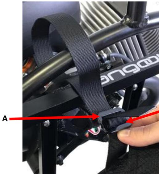
3 : Loop back around the hoop and insert the strap into A.
