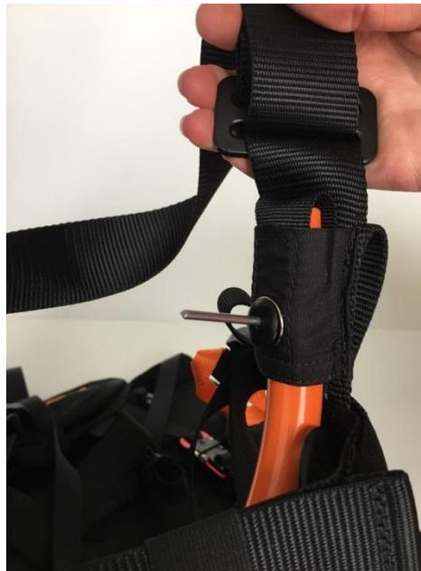
3: Place the rivet as shown and then set it with the riveting machine.
