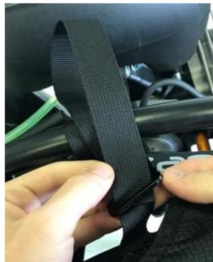
4 : Insert the strap into B without tightening it (see picture 4).
