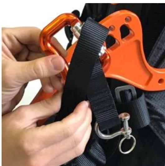
3 : Make a buckle loop with the connecting strap around the horizontal strap.
