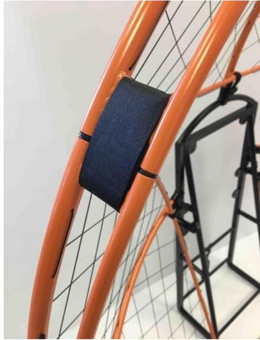
2 : Insert the top cage section in the top right and left ones and attach the Velcro straps as shown
