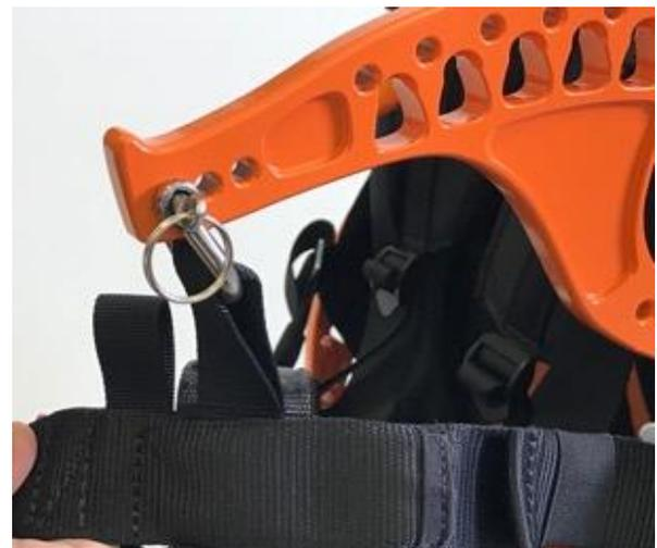
4 : Connect the previous shackle to the top of the swan neck arm (adjustment depend on the weight and comfort of the pilot).
