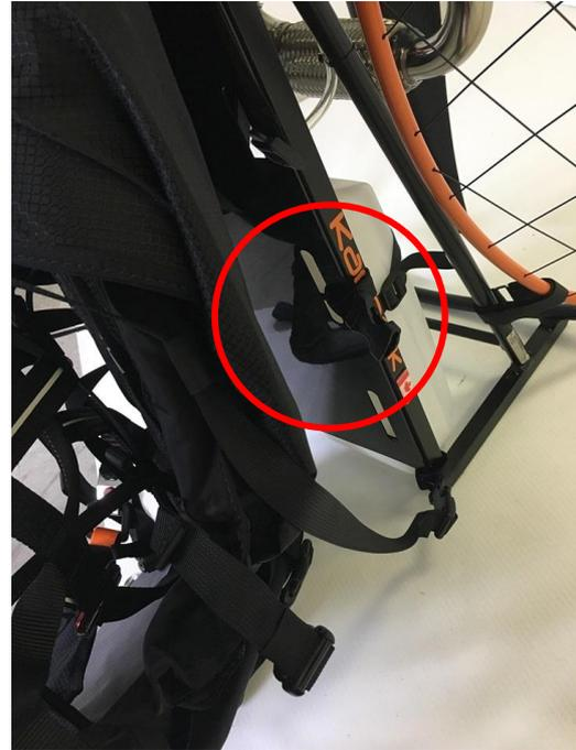
2: Unfasten the quick release buckle then attach it at the specified location.
