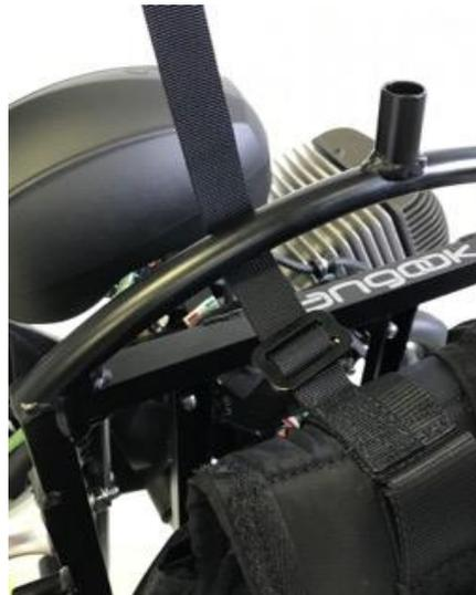
2 : Place the harness against the frame and pass the strap under the hoop.
