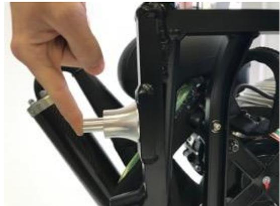
Result: Be careful to attach the, left and right connectors based on the counter balance requirement for your specific engine type. Direct drive motors pull to the left while belt drive motors pull to the right.:
