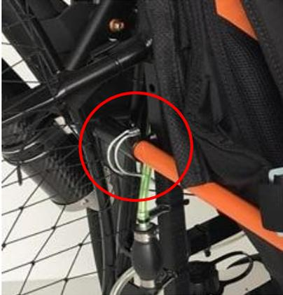
*Fix the bars on the frame by means of shackles.*
