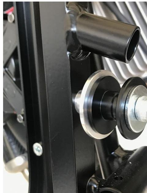
3 : Keep on drilling until you are able to insert the connector. Repeat the step on the other side of the frame.
