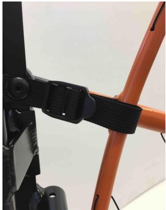
8 : Finally, tighten the strap and any cut excess. Be sure to leave at least 5cm.
