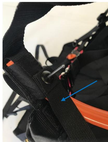
4 : Put the end of the arm in the designed compartment, then position the blocking strap (blue arrow) and fix using a rivet.
