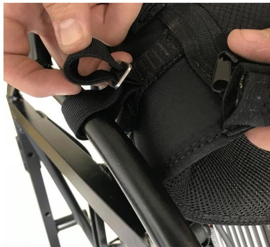
4 : Pull the strap through the second buckle, do not over tighten.
