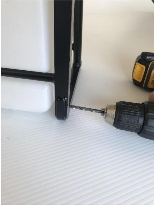
1 : Make a mark 2 cm above the bottom of the frame. Use the 13/64" drill bit to pierce only the first surface of the bar. **It is useless to fully drill the bar.**
