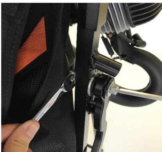
3 : Tighten with the 13 mm spanner and the 6 mm Allen key. Do it on both sides.
