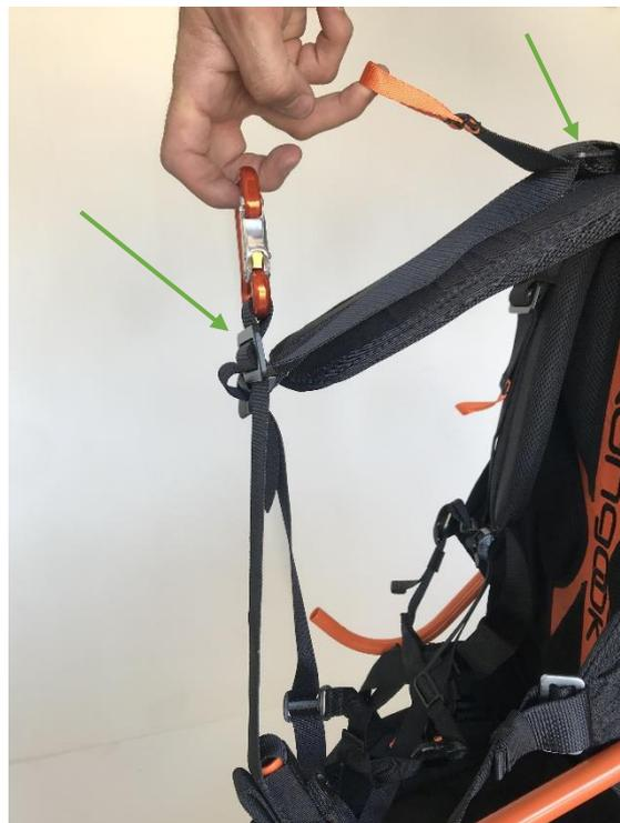
11 : To calibrate the paramotor, adjust the straps thanks to the two buckles (green arrows). For more information about calibration, refer to page 23 (Hang test).
