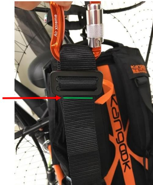
3: Once the definitive position of the buckle is chosen, mark it. Then, remove the carabiner and the buckle.
